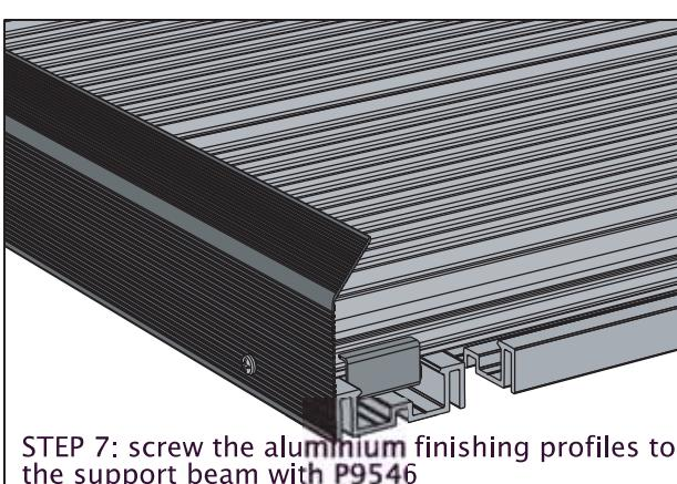
STEP 7: screw the aluminium finishing profiles to the support beam with P9546
